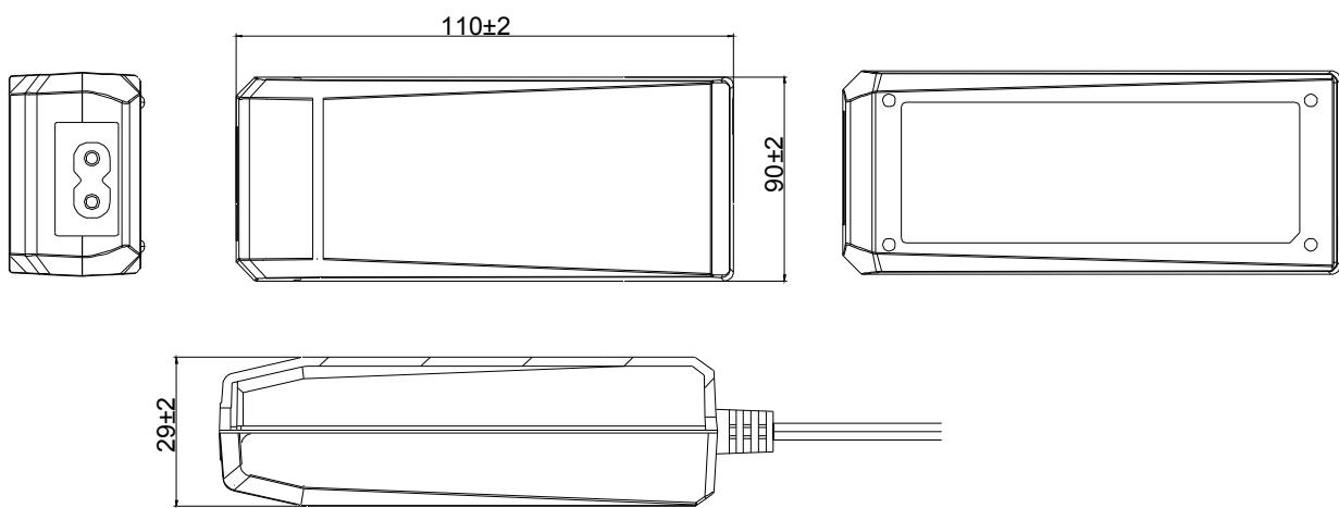
All Dimensions are in mm, Tolerance: X.X±0.5
